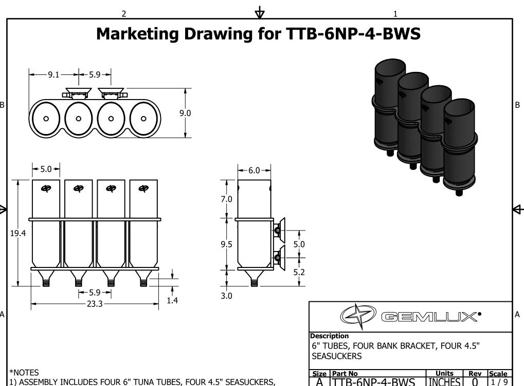
1) ASSEMBLY INCLUDES FOUR 6" TUNA TUBES, FOUR 4.5" SEASUCKERS, FOUR NOSE CONES, AND BRACKET ONLY.
