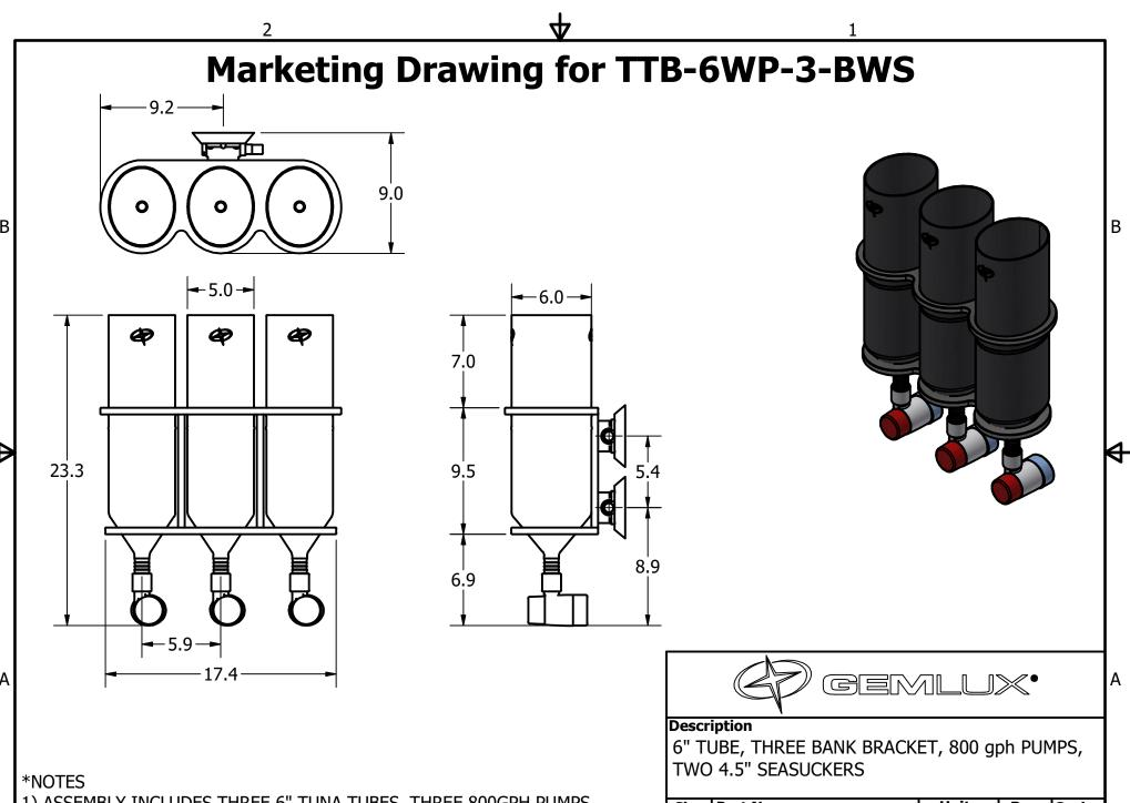
1) ASSEMBLY INCLUDES THREE 6" TUNA TUBES, THREE 800GPH PUMPS, TWO 4.5" SEASUCKERS, THREE NOSE CONES, AND BRACKET.
